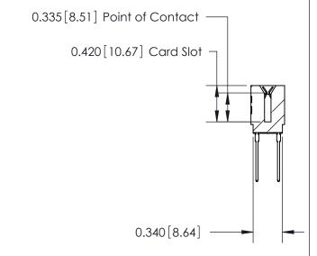
ACAD REFERENCE NO. 726 Series Ultra-Mate Card Edge Connector - Press Fit DRAWN: Part Number: 726-020-545-201 CHECKED: **EDAC INC** SCALE: THESE DRAWINGS AND SPECIFICATIONS ARE THE PROPERTY OF EDAC INC.,AND TORONTO, ONTARIO SHALL NOT BE REPRODUCED, OR COPIED CANADA
