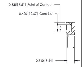
726 Series Ultra-Mate Card Edge Connector - Press Fit
