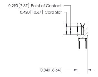
726 Series Ultra-Mate Card Edge Connector - Press Fit Part Number: 726-016-527-201 **EDAC INC** THESE DRAWINGS AND SPECIFICATIONS ARE THE PROPERTY OF EDAC INC.,AND TORONTO, ONTARIO SHALL NOT BE REPRODUCED, OR COPIED CANADA OR USED AS THE BASIS FOR THE MANUFACTURE OR SALE OF APPARATUS YOUR CONNECTION TO QUALITY & SERVICE WITHOUT WRITTEN PERMISSION.
