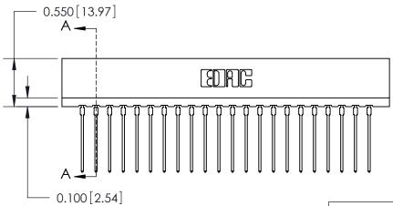
717 Series Ultra-Mate Card Edge Connector - Press Fit Part Number: 717-044-541-201
