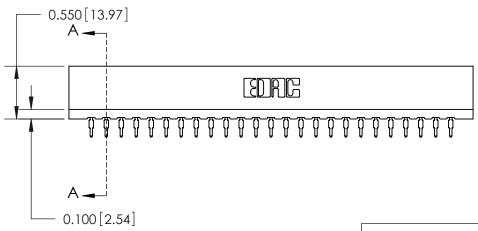
0.420 [10.67] Card Slot 0.34 [8.53] 0.31 7.77 Point of Contact 0.550 13.97 0.300 [7.62] SECTION A-A
