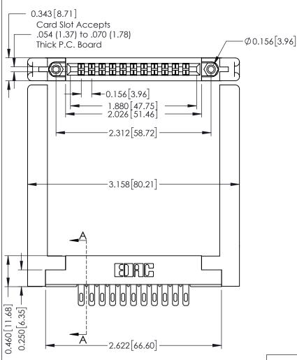
SECTION 0.295 [7.49] Card Slot 0.165[4.19] Point of Contact
