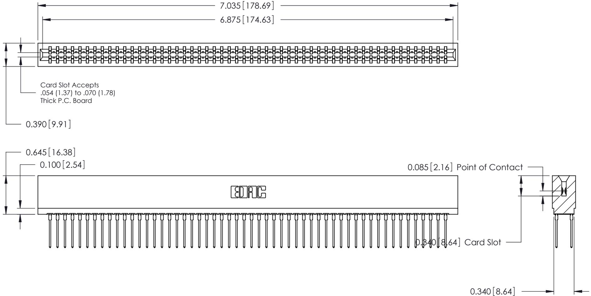
746 Series Ultra-Mate Card Edge Connector - Press Fit
