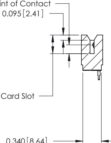
746 Series Ultra-Mate Card Edge Connector - Press Fit
