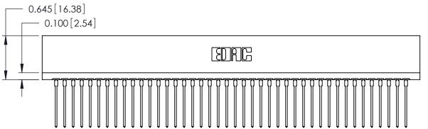
746 Series Ultra-Mate Card Edge Connector - Press Fit
