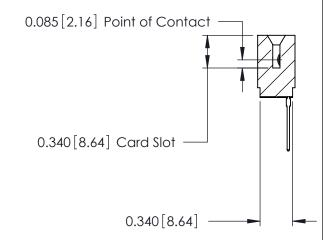
746 Series Ultra-Mate Card Edge Connector - Press Fit Part Number: 746-040-540-501 **EDAC INC** THESE DRAWINGS AND SPECIFICATIONS
