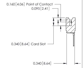
746 Series Ultra-Mate Card Edge Connector - Press Fit Part Number: 746-034-545-506 **EDAC INC** THESE DRAWINGS AND SPECIFICATIONS ARE THE PROPERTY OF EDAC INC.,AND TORONTO, ONTARIO SHALL NOT BE REPRODUCED, OR COPIED CANADA OR USED AS THE BASIS FOR THE
