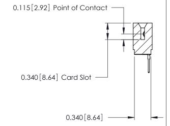
746 Series Ultra-Mate Card Edge Connector - Press Fit Part Number: 746-032-527-501 **EDAC INC** THESE DRAWINGS AND SPECIFICATIONS ARE THE PROPERTY OF EDAC INC.,AND TORONTO, ONTARIO SHALL NOT BE REPRODUCED, OR COPIED CANADA
