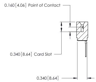
ACAD REFERENCE NO. 746-ENG MASTER 746 Series Ultra-Mate Card Edge Connector - Press Fit DRAWN: DATE: AUG 20/09 J.LEE Part Number: 746-015-545-501 CHECKED: DATE: **EDAC INC** SCALE: SHEET 1 OF 1 THESE DRAWINGS AND SPECIFICATIONS ARE THE PROPERTY OF EDAC INC.,AND TORONTO, ONTARIO SHALL NOT BE REPRODUCED, OR COPIED DRAWING NUMBER CANADA OR USED AS THE BASIS FOR THE 746-ENG MASTER MANUFACTURE OR SALE OF APPARATUS YOUR CONNECTION TO QUALITY & SERVICE WITHOUT WRITTEN PERMISSION.
