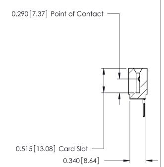
ACAD REFERENCE NO. 746-ENG MASTER 746 Series Ultra-Mate Card Edge Connector - Press Fit DRAWN: J.LEE DATE: AUG 20/09 Part Number: 746-011-527-101 CHECKED: DATE: **EDAC INC** SCALE: SHEET 1 OF 1 THESE DRAWINGS AND SPECIFICATIONS ARE THE PROPERTY OF EDAC INC.,AND TORONTO, ONTARIO SHALL NOT BE REPRODUCED, OR COPIED DRAWING NUMBER CANADA OR USED AS THE BASIS FOR THE 746-ENG MASTER MANUFACTURE OR SALE OF APPARATUS YOUR CONNECTION TO QUALITY & SERVICE WITHOUT WRITTEN PERMISSION.
