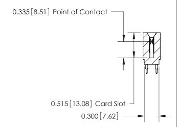
ACAD REFERENCE NO. 745 Series Ultra-Mate Card Edge Connector - Press Fit DRAWN: DATE: MAY 04/09 J.LEE Part Number: 745-066-525-201 CHECKED: DATE: **EDAC INC** SCALE: SHEET 1 OF 2 THESE DRAWINGS AND SPECIFICATIONS ARE THE PROPERTY OF EDAC INC.,AND TORONTO, ONTARIO SHALL NOT BE REPRODUCED, OR COPIED DRAWING NUMBER CANADA OR USED AS THE BASIS FOR THE 745-ENG MASTER MANUFACTURE OR SALE OF APPARATUS YOUR CONNECTION TO QUALITY & SERVICE WITHOUT WRITTEN PERMISSION.
