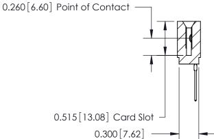
745 Series Ultra-Mate Card Edge Connector - Press Fit Part Number: 745-054-540-101
