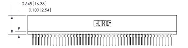
745 Series Ultra-Mate Card Edge Connector - Press Fit
