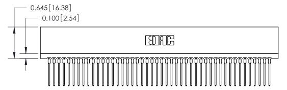
745 Series Ultra-Mate Card Edge Connector - Press Fit
