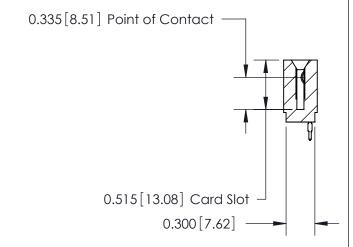
ACAD REFERENCE NO. 745 Series Ultra-Mate Card Edge Connector - Press Fit DRAWN: J.LEE Part Number: 745-046-525-101 CHECKED: **EDAC INC** SCALE: THESE DRAWINGS AND SPECIFICATIONS ARE THE PROPERTY OF EDAC INC.,AND TORONTO, ONTARIO SHALL NOT BE REPRODUCED, OR COPIED DRAWING NUMBER CANADA OR USED AS THE BASIS FOR THE 745-ENG MASTER MANUFACTURE OR SALE OF APPARATUS YOUR CONNECTION TO QUALITY & SERVICE WITHOUT WRITTEN PERMISSION.
