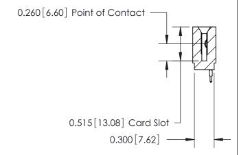
ACAD REFERENCE NO. 745 Series Ultra-Mate Card Edge Connector - Press Fit DRAWN: J.LEE Part Number: 745-043-520-101 CHECKED: SCALE: **EDAC INC** THESE DRAWINGS AND SPECIFICATIONS ARE THE PROPERTY OF EDAC INC.,AND TORONTO, ONTARIO SHALL NOT BE REPRODUCED, OR COPIED DRAWING NUMBER OR USED AS THE BASIS FOR THE CANADA 745-ENG MASTER MANUFACTURE OR SALE OF APPARATUS YOUR CONNECTION TO QUALITY & SERVICE WITHOUT WRITTEN PERMISSION.
