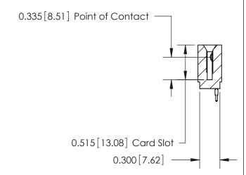
ACAD REFERENCE NO. 745 Series Ultra-Mate Card Edge Connector - Press Fit DRAWN: J.LEE Part Number: 745-040-525-101 CHECKED: **EDAC INC** SCALE: THESE DRAWINGS AND SPECIFICATIONS ARE THE PROPERTY OF EDAC INC.,AND TORONTO, ONTARIO SHALL NOT BE REPRODUCED, OR COPIED DRAWING NUMBER CANADA OR USED AS THE BASIS FOR THE 745-ENG MASTER MANUFACTURE OR SALE OF APPARATUS YOUR CONNECTION TO QUALITY & SERVICE WITHOUT WRITTEN PERMISSION.
