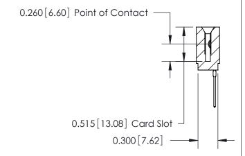
ACAD REFERENCE NO. 745 Series Ultra-Mate Card Edge Connector - Press Fit DRAWN: J.LEE Part Number: 745-015-540-101 CHECKED: SCALE: **EDAC INC** THESE DRAWINGS AND SPECIFICATIONS ARE THE PROPERTY OF EDAC INC.,AND TORONTO, ONTARIO SHALL NOT BE REPRODUCED, OR COPIED DRAWING NUMBER CANADA OR USED AS THE BASIS FOR THE 745-ENG MASTER MANUFACTURE OR SALE OF APPARATUS YOUR CONNECTION TO QUALITY & SERVICE WITHOUT WRITTEN PERMISSION.
