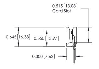
ACAD REFERENCE NOTION STEP 737 Series Ultra-Mate Card Edge Connector - Press Fit DRAWN: Part Number: 737-015-545-106 CHECKED: **EDAC INC** THESE DRAWINGS AND SPECIFICATIONS ARE THE PROPERTY OF EDAC INC.,AND TORONTO, ONTARIO SHALL NOT BE REPRODUCED, OR COPIED CANADA OR USED AS THE BASIS FOR THE
