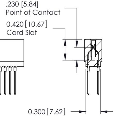
725 Series Ultra-Mate Card Edge Connector - Press Fit
