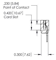
ACAD REFERENCE NOS EGALONISARA 725 Series Ultra-Mate Card Edge Connector - Press Fit DRAWN: Part Number: 725-033-522-101 CHECKED: **EDAC INC** THESE DRAWINGS AND SPECIFICATIONS ARE THE PROPERTY OF EDAC INC.,AND TORONTO, ONTARIO SHALL NOT BE REPRODUCED, OR COPIED CANADA OR USED AS THE BASIS FOR THE
