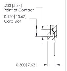
725 Series Ultra-Mate Card Edge Connector - Press Fit Part Number: 725-023-540-101
