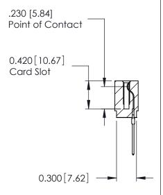
ACAD REFERENCE NO. 725-ENG MASTER 725 Series Ultra-Mate Card Edge Connector - Press Fit SEGAHON:3A:9A DRAWN: J.LEE Part Number: 725-017-545-101 CHECKED: DATE: **EDAC INC** SCALE: SHEET 1 OF 1 THESE DRAWINGS AND SPECIFICATIONS ARE THE PROPERTY OF EDAC INC.,AND TORONTO, ONTARIO SHALL NOT BE REPRODUCED, OR COPIED DRAWING NUMBER **ISSUE** CANADA OR USED AS THE BASIS FOR THE 725-ENG MASTER MANUFACTURE OR SALE OF APPARATUS YOUR CONNECTION TO QUALITY & SERVICE WITHOUT WRITTEN PERMISSION.
