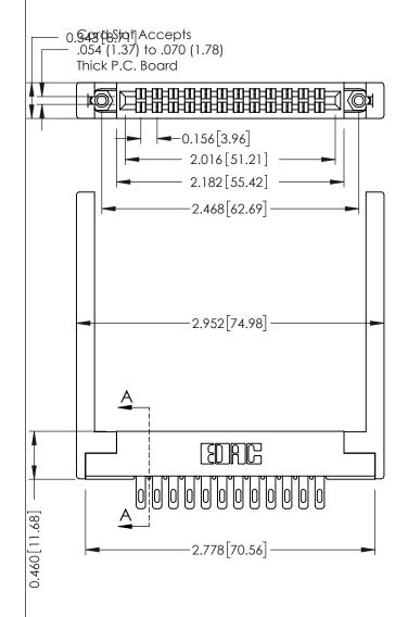
0.295[7.49] Card Slot SECTION 0.090 [2.29] Point of Contact 305 ENG MASTER 305 / 315 / 355 Card Edge Connector
