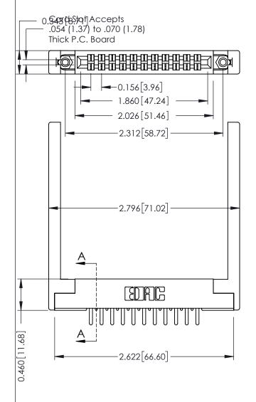
**ECTION A-A** 0.295[7.49] Card Slot 0.090[2.29] Point of Contact 305 ENG MASTER
