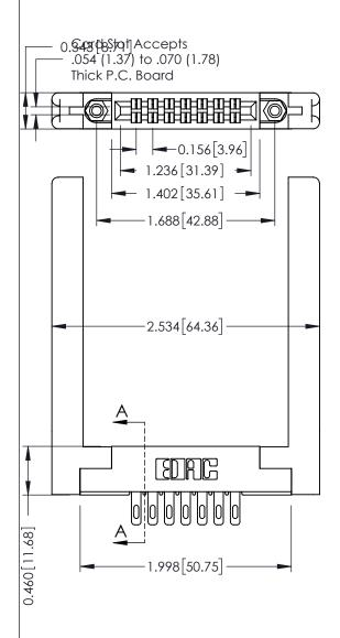
0.090[2.29] Point of Contact 305 ENG MASTER 305 / 315 / 355 Card Edge Connector J.LEE DATE: SEPT. 21/09 Part Number: 315-014-500-258 NTS SHEET 1 OF 2
