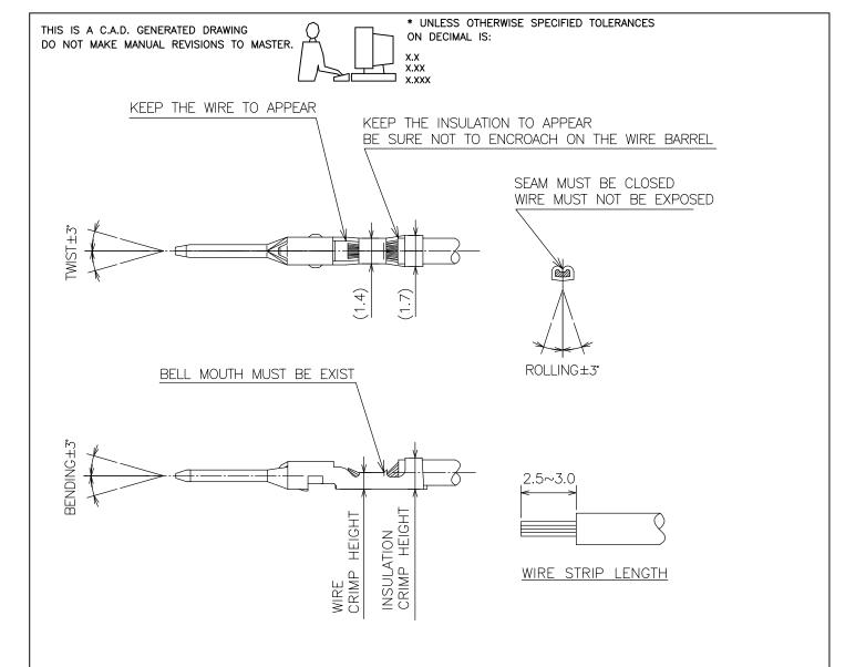
WIRE CRIMP INFORMATION FOR 565-290-731 CONTACT WITH INSULATION DIA 1.3mm TO 1.7mm (565-290-731 CONTACT TO BE CRIMPED WITH TOOL# 565-280-211)
