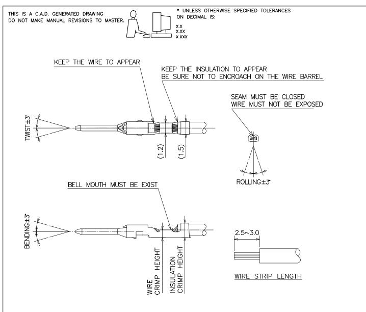
WIRE CRIMP INFORMATION FOR 565-290-711 CONTACT WITH INSULATION DIA 1.0mm TO 1.3mm (565-290-711 CONTACT TO BE CRIMPED WITH TOOL# 565-280-210)
