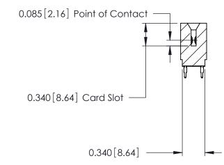
ACAD REFERENCE NO. 746-ENG MASTER 746 Series Ultra-Mate Card Edge Connector - Press Fit DRAWN: J.LEE DATE: AUG 20/09 Part Number: 746-076-520-601 CHECKED: DATE: **EDAC INC** SCALE: SHEET 1 OF 1 THESE DRAWINGS AND SPECIFICATIONS ARE THE PROPERTY OF EDAC INC.,AND TORONTO, ONTARIO SHALL NOT BE REPRODUCED, OR COPIED DRAWING NUMBER
