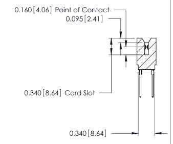
ACAD REFERENCE NO. 746 Series Ultra-Mate Card Edge Connector - Press Fit DRAWN: Part Number: 746-074-545-606 CHECKED: **EDAC INC** THESE DRAWINGS AND SPECIFICATIONS ARE THE PROPERTY OF EDAC INC.,AND TORONTO, ONTARIO SHALL NOT BE REPRODUCED, OR COPIED CANADA
