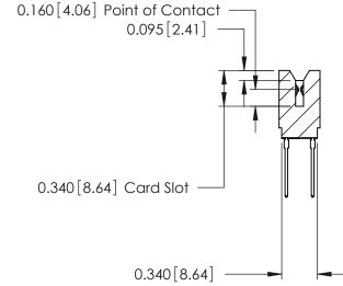
ACAD REFERENCE NO. 746 Series Ultra-Mate Card Edge Connector - Press Fit DRAWN: J.LEE Part Number: 746-064-545-606 CHECKED: **EDAC INC** SCALE: THESE DRAWINGS AND SPECIFICATIONS ARE THE PROPERTY OF EDAC INC.,AND TORONTO, ONTARIO SHALL NOT BE REPRODUCED, OR COPIED DRAWING NUMBER CANADA OR USED AS THE BASIS FOR THE 746-ENG MASTER MANUFACTURE OR SALE OF APPARATUS YOUR CONNECTION TO QUALITY & SERVICE WITHOUT WRITTEN PERMISSION.
