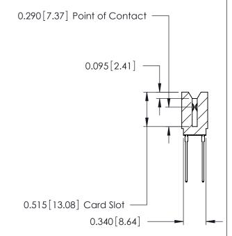
746 Series Ultra-Mate Card Edge Connector - Press Fit ACAD REFERENCE NO.
