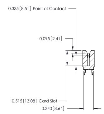
ACAD REFERENCE NO. 746 Series Ultra-Mate Card Edge Connector - Press Fit DRAWN: J.LEE Part Number: 746-056-525-206 CHECKED: **EDAC INC** SCALE: THESE DRAWINGS AND SPECIFICATIONS ARE THE PROPERTY OF EDAC INC.,AND TORONTO, ONTARIO SHALL NOT BE REPRODUCED, OR COPIED CANADA
