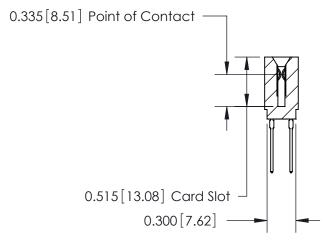
745 Series Ultra-Mate Card Edge Connector - Press Fit Part Number: 745-104-545-201
