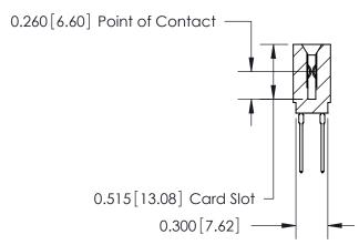
745 Series Ultra-Mate Card Edge Connector - Press Fit Part Number: 745-104-540-201 **EDAC INC** THESE DRAWINGS AND SPECIFICATIONS ARE THE PROPERTY OF EDAC INC.,AND TORONTO, ONTARIO SHALL NOT BE REPRODUCED, OR COPIED CANADA
