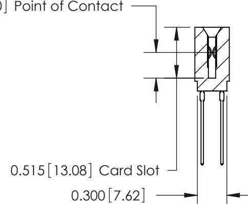
745 Series Ultra-Mate Card Edge Connector - Press Fit
