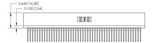
745 Series Ultra-Mate Card Edge Connector - Press Fit
