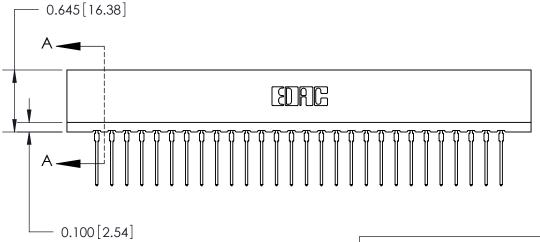
737 Series Ultra-Mate Card Edge Connector - Press Fit
