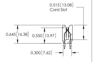
737 Series Ultra-Mate Card Edge Connector - Press Fit ACAD REFERENCE NO.
