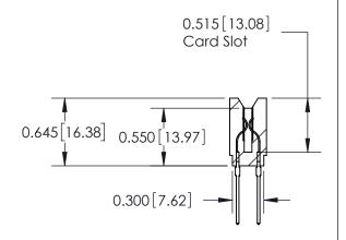
737 Series Ultra-Mate Card Edge Connector - Press Fit ACAD REFERENCE @TION - ACAD REFERENCE
