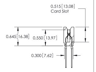
ACAD REFERENCE NO. 737 Series Ultra-Mate Card Edge Connector - Press Fit DRAWN: Part Number: 737-030-541-206 CHECKED: **EDAC INC** SCALE: THESE DRAWINGS AND SPECIFICATIONS ARE THE PROPERTY OF EDAC INC.,AND TORONTO, ONTARIO SHALL NOT BE REPRODUCED, OR COPIED DRAWING NUMBER CANADA OR USED AS THE BASIS FOR THE MANUFACTURE OR SALE OF APPARATUS YOUR CONNECTION TO QUALITY & SERVICE WITHOUT WRITTEN PERMISSION.
