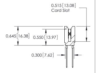
ACAD REFERENCE NO. 737 Series Ultra-Mate Card Edge Connector - Press Fit DRAWN: Part Number: 737-020-541-206 CHECKED: **EDAC INC** SCALE: THESE DRAWINGS AND SPECIFICATIONS ARE THE PROPERTY OF EDAC INC.,AND TORONTO, ONTARIO SHALL NOT BE REPRODUCED, OR COPIED DRAWING NUMBER CANADA OR USED AS THE BASIS FOR THE MANUFACTURE OR SALE OF APPARATUS YOUR CONNECTION TO QUALITY & SERVICE WITHOUT WRITTEN PERMISSION.
