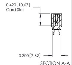
725 Series Ultra-Mate Card Edge Connector - Press Fit
