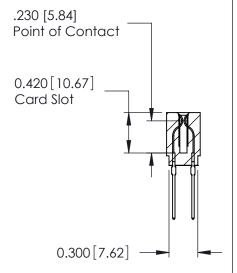
ACAD REFERENCE NO. 725-ENG MASTER 725 Series Ultra-Mate Card Edge Connector - Press Fit SEGAHON:3A:9A DRAWN: J.LEE Part Number: 725-042-545-201 CHECKED: DATE: SCALE: **EDAC INC** SHEET 1 OF 1 THESE DRAWINGS AND SPECIFICATIONS ARE THE PROPERTY OF EDAC INC.,AND TORONTO, ONTARIO SHALL NOT BE REPRODUCED, OR COPIED DRAWING NUMBER **ISSUE** CANADA OR USED AS THE BASIS FOR THE 725-ENG MASTER MANUFACTURE OR SALE OF APPARATUS YOUR CONNECTION TO QUALITY & SERVICE WITHOUT WRITTEN PERMISSION.
