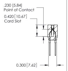
ACAD REFERENCE NO. 725 Series Ultra-Mate Card Edge Connector - Press Fit DRAWN: Part Number: 725-036-540-201 CHECKED: **EDAC INC** THESE DRAWINGS AND SPECIFICATIONS ARE THE PROPERTY OF EDAC INC.,AND
