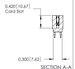
725 Series Ultra-Mate Card Edge Connector - Press Fit ACAD REFERENCE NO.
