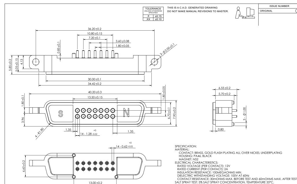
MAGNETIC SPRING LOADED CONNECTOR, 14POS, FEMALE
